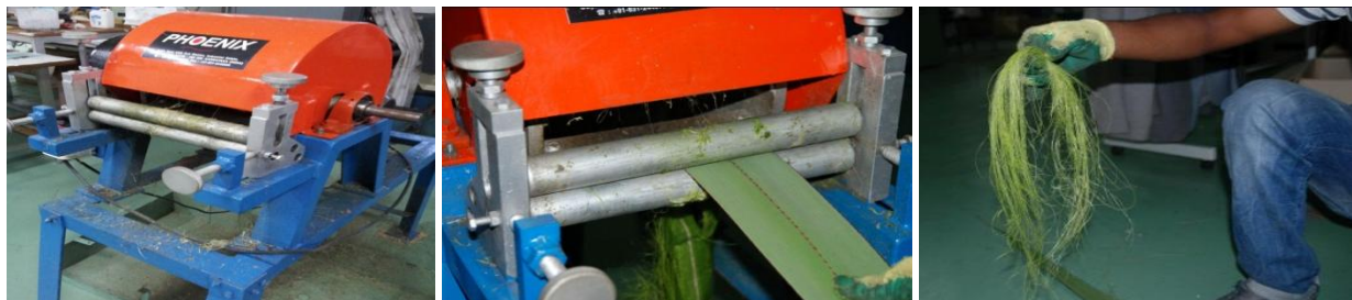
Figure 6: Modified raspador fibre extraction machine for Pandanus utilis leaves
